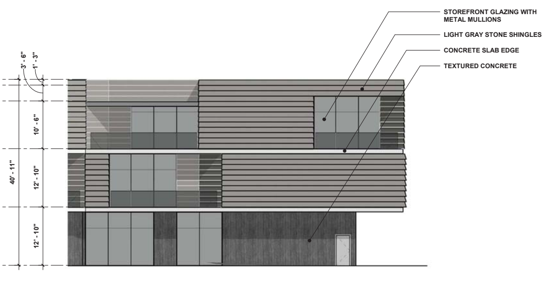
2 Elevation - Building C - West 1
